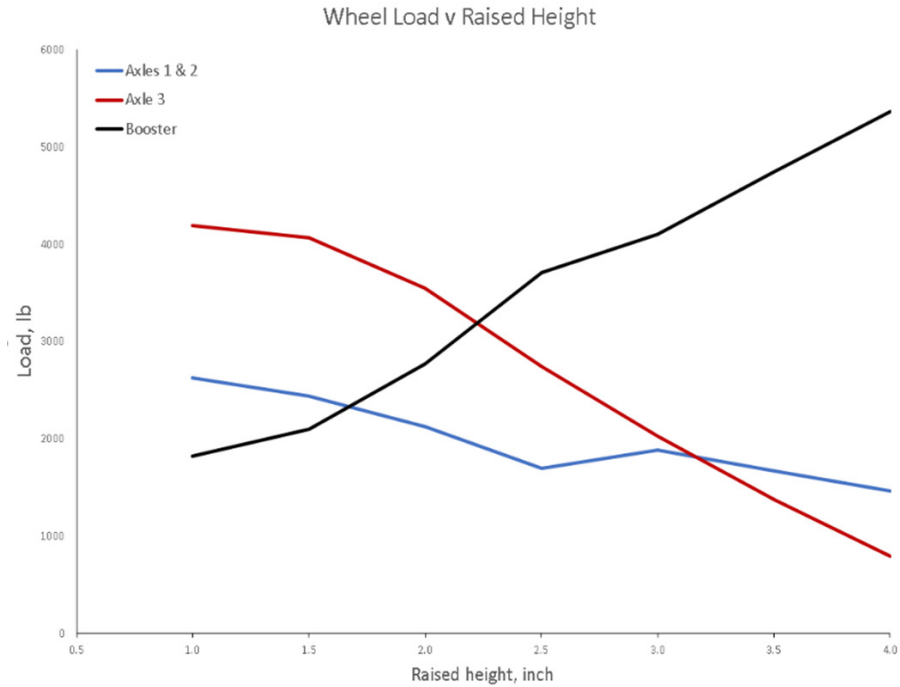
Figure 8 Wheel load as a function of raised height of tractor-booster axle datum.
