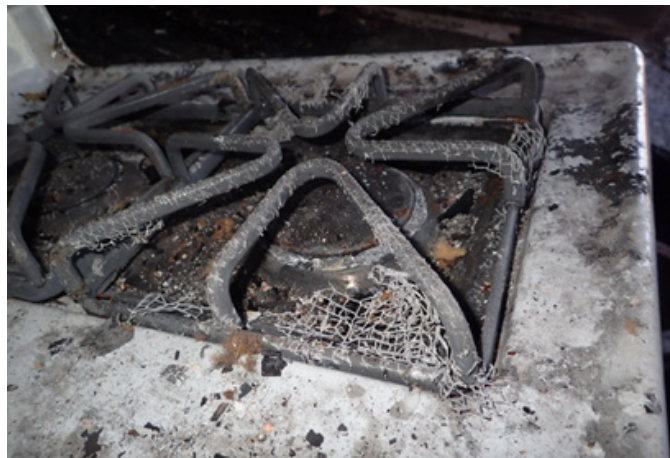
Figure 9 Mesh found on right-front burner.
