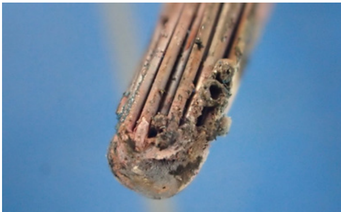
Figure 2 Arc site found at the fire scene.
