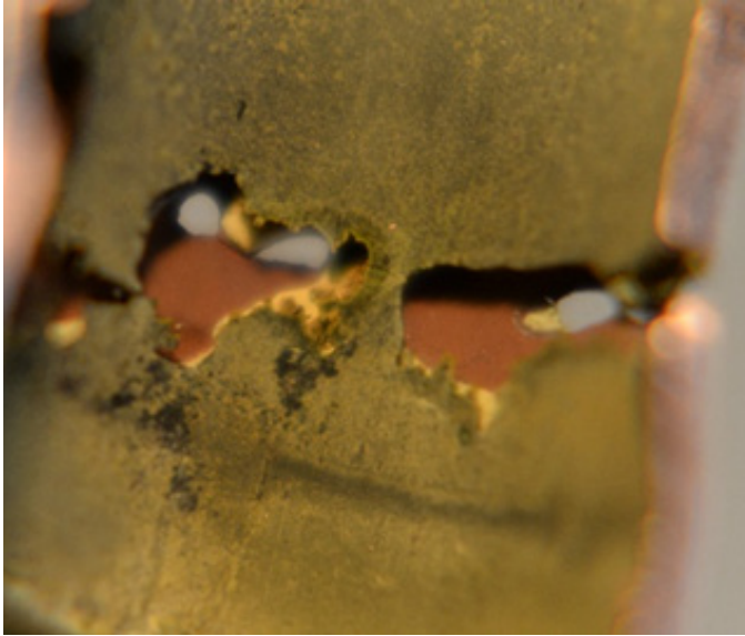
Figure 7 Erosion penetrations at poorly formed joints.
