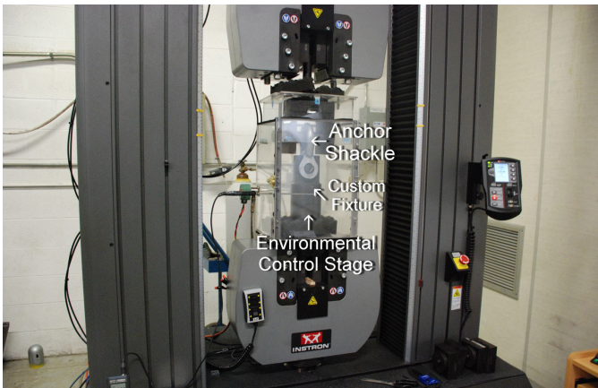
Figure 17 Environmental control stage on the Instron tensile test machine for rated load tests.
