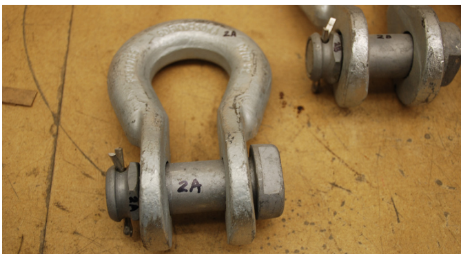
Figure 1 Typical Number 9 anchor shackle with clevis pin.
