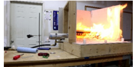
Figure 14g Flash fire propagation right to left.
