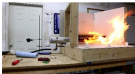
Figure 14f Flash fire propagation right to left.
