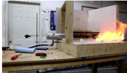
Figure 14d Flash fire propagates into the firebox.
