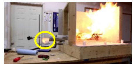
Figure 14i Flash fire propagation through and out rigid duct work.
