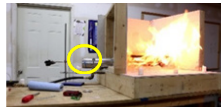
Figure 14h Pressure wave ahead of the flame front distorts the candle flame (circled).
