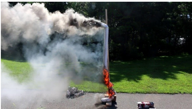
Figure 13c Rapid upward flame spread.
