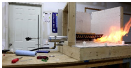
Figure 14e Flash fire propagation into the firebox.
