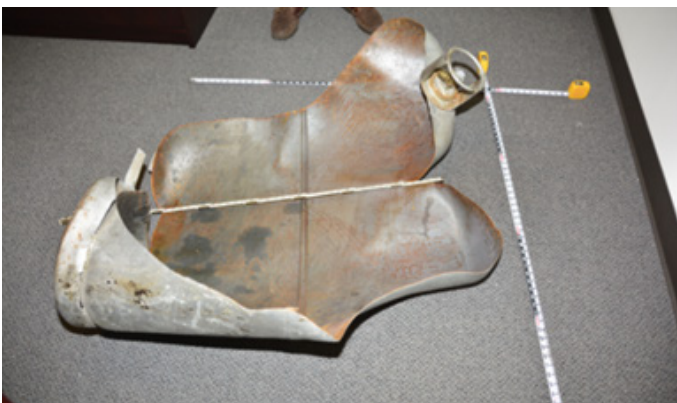
Figure 15 Left cylinder. The cylinder was ruptured, and the cylinder valve had no relief valve or fixed maximum liquid level gauge.
