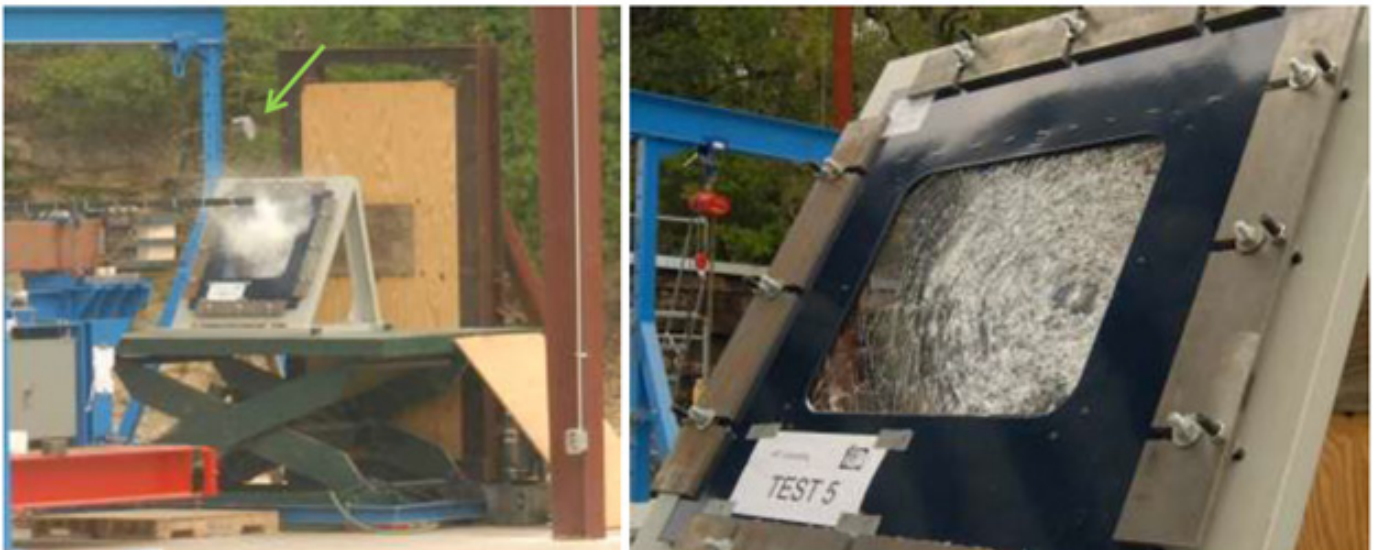
Figure 11 Test 5 – European market CNC lathe window using 12-mm polycarbonate pane.
