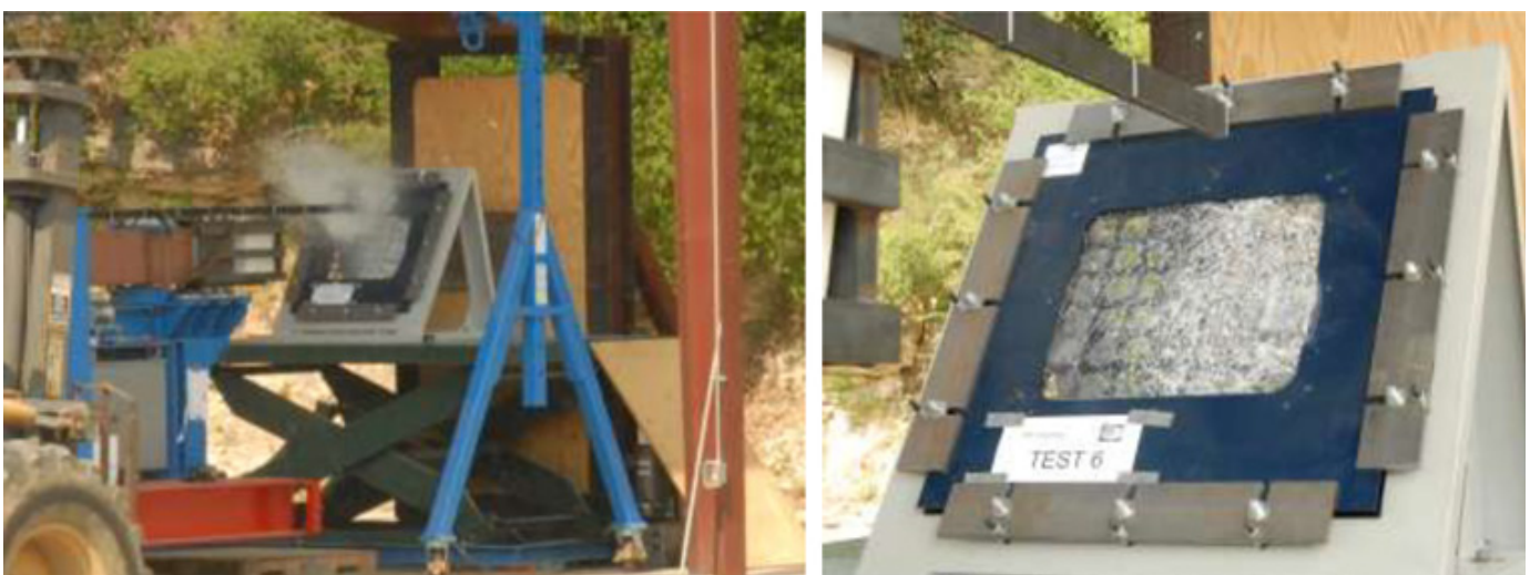
Figure 12 Test 6 – “Maximum Protection” CNC lathe window using muntin bars at exterior surface.
