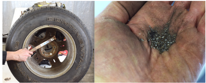
Figure 13 Debris from a wheel after it was removed from an SUV with a wire brush.
