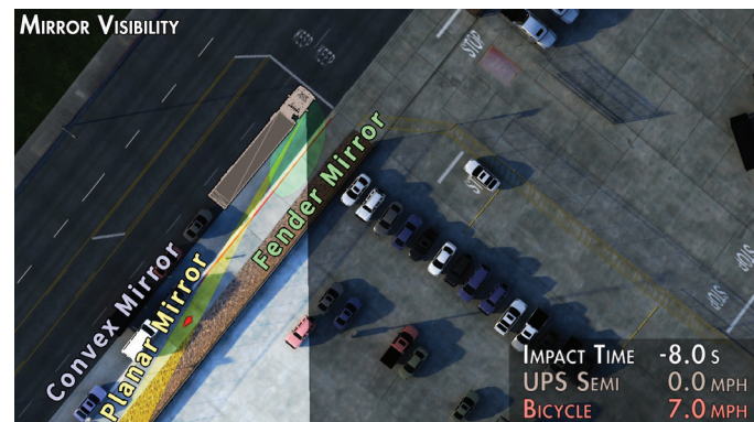
Figure 30 Visibility cones created for the three mirrors 8 seconds before impact.
