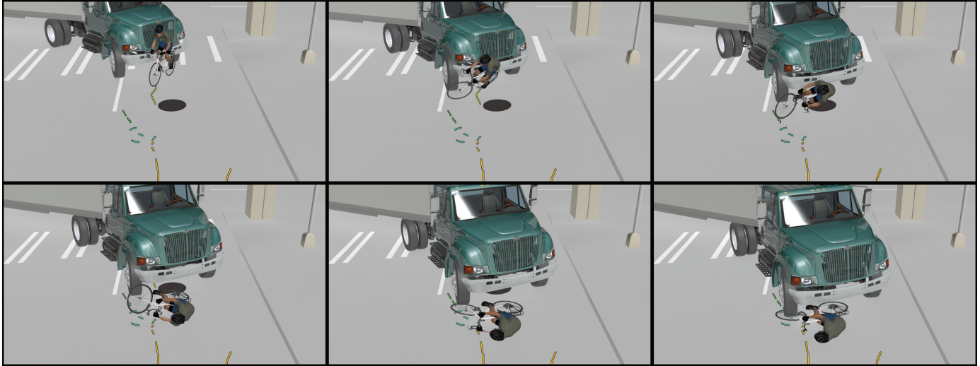
Figure 12 Impact progression of bicycle and rider based on PC-Crash simulation.
