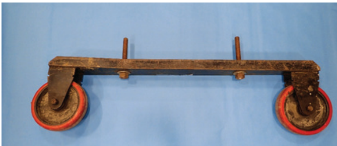
Figure 24 Damaged wheel frame.
