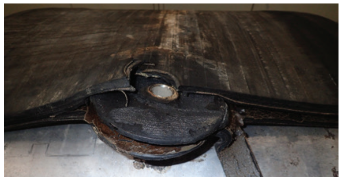
Figure 18 Bladder rupture at test cavity fill tube.
