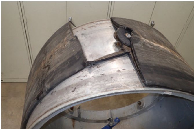
Figure 14 Top of joint tester showing ruptured bladder.
