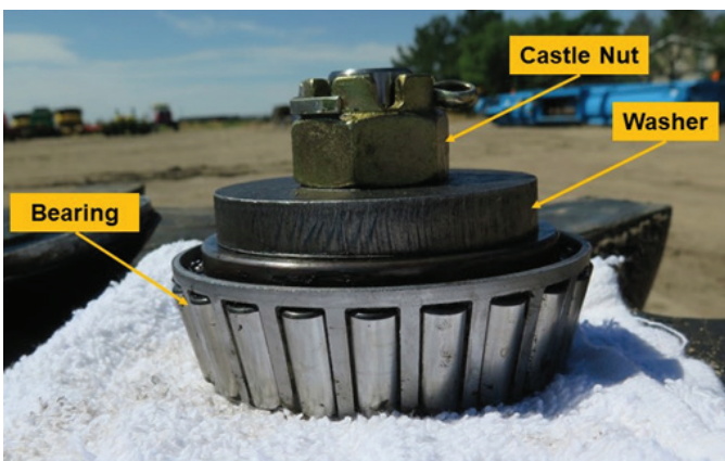
Figure 19 Assembly of the tapered bearing, washer, and castle nut.
