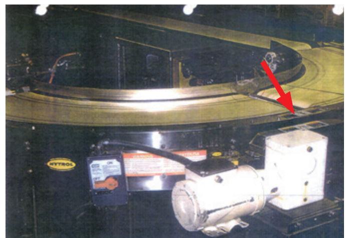
Figure 3 Arrow shows where worker was injured between two 90° conveyor sections while removing cookie nuggets from the conveyor. Product flows from left to right.
