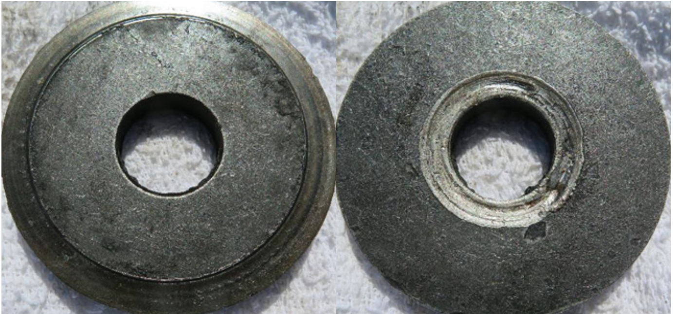
Figure 18 Washer bearing side (left), nut side (right).
