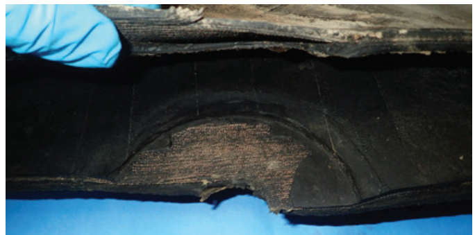
Figure 17 Bladder reinforcing cords.
