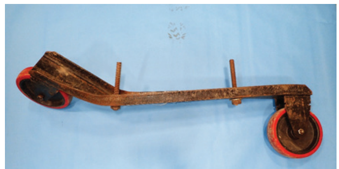
Figure 23 Damaged wheel frame.
