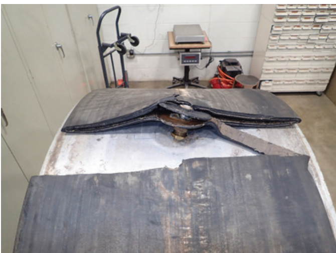
Figure 15 Ruptured bladder showing test cavity supply tube connection.
