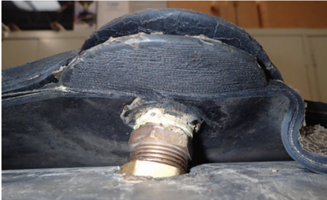
Figure 19 Bladder rupture at test cavity fill tube.
