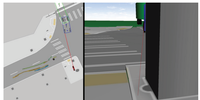
Figure 14 2D line-of-sight (left) and 3D line-of-sight in PC-Crash.
