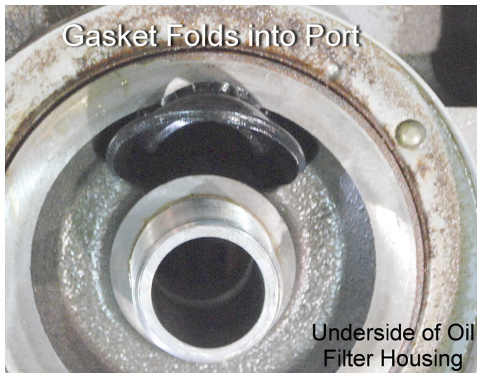
Figure 31 Gasket folded into port demonstration.
