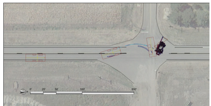
Figure 8 Motion of the combine prior to rest along the physical evidence.
