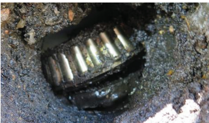
Figure 13 View inside left rear steering knuckle showing spindle components and grease.
