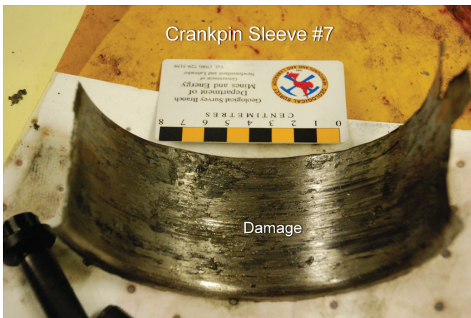
Figure 4 Shell damage on rod cap for cylinder #7.
