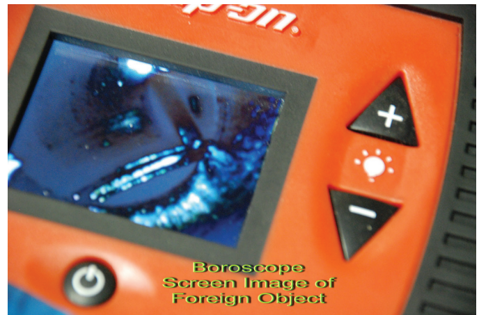
Figure 21 Boroscope screen image with foreign object.
