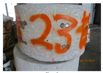
Figure 8 Concrete core with excessive flexural cracking.
