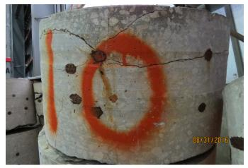
Figure 9 Concrete core with horizontal cracking.
