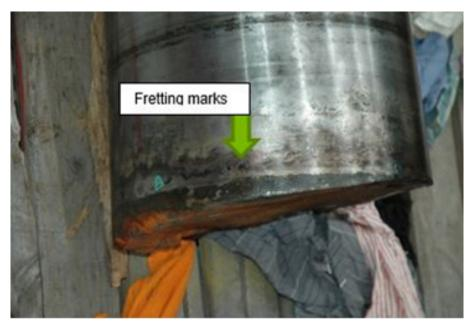
Figure 5 Fretting marks on the shaft stub.
