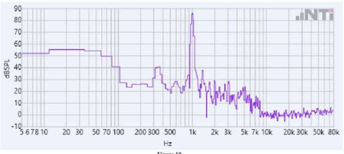
Figure 10 The partially designed system buyer's system output spectrum with 1 kHz input.
