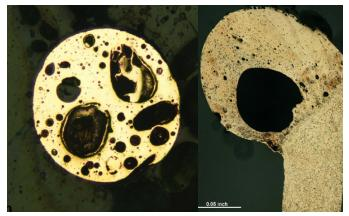
Figure 3 Arc sites to copper conductors.
