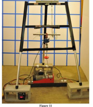
Load test set-up. Load is applied through wire rope (with load cell) to spreader bar, then to loading bar strapped to top scaffold brace.
