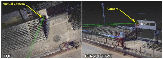
Figure 9 Top view (left) and perspective view (right) of the motorsports park grandstands showing the location of the virtual camera solved by matchmoving.
