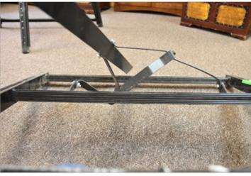
Figure 5 Two overall views of failed scaffold support with legs collapsed. Note the fractured lug welds at top of left image and deformation of spreader bar assembly visible in both views.
