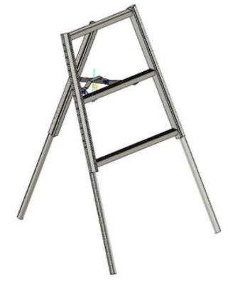
Figure 6 Overall view of basic model used for finite element analysis.
