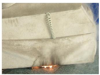
**Figure 7** Ignition of fabric by glowing power cord.
