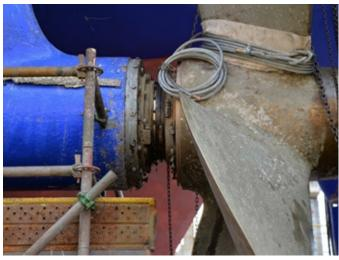
Figure 3 The fracture in the starboard shaft occurred just inside the propeller hub.
