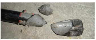
**Figure 15** A typical torque failure.
