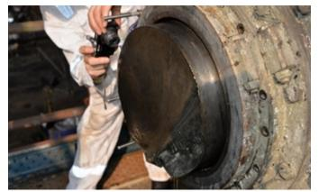
Figure 9 The fracture face on the tail shaft after removal of the protective cap.
