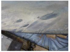
Figure 7 Cavitation erosion caused by small indentations and poor edge form to the leading edge.
