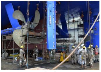
Figure 2 The port side arrangement is similar. In this photo, the new highefficiency propeller is in place and rudder is inclined toward the camera.
