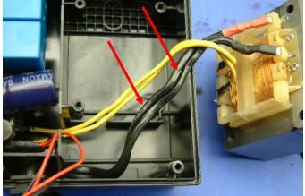
Figure 3 Wiring connections in the older design show evidence of external force (red arrows).
