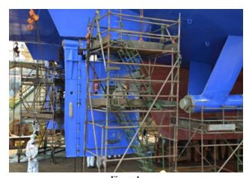
Figure 1 Arrangement of shaft, propeller, and rudder. The exposed shaft end is where the starboard propeller was mounted before it was lost.
