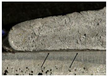
Figure 3 Photomicrograph from the plaintiff's expert's preliminary report, highlighting lack of root penetration.
