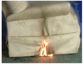
Figure 8 Propagation of fire to fabric.
