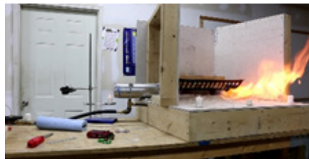
Figure 14e Flash fire propagation into the firebox.
