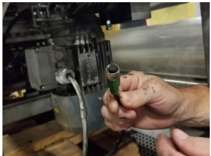
Figure 13 Opposite end of the cable of Figure 10 where it attaches to the microprocessor.
