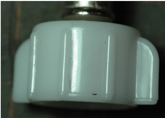
Figure 11 Before torque to failure — no tool marks.
