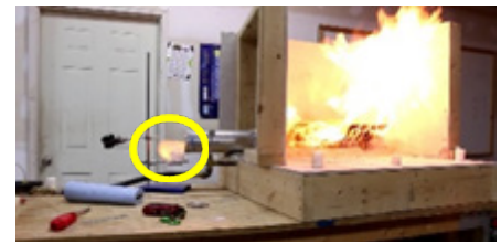
Figure 14i Flash fire propagation through and out rigid duct work.
