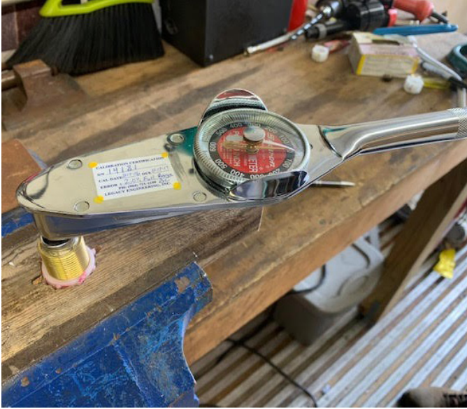
Figure 10 Torque wrench and nut in wood block.
