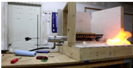
Figure 14c Flash fire initiated at right-hand side safety candle.
