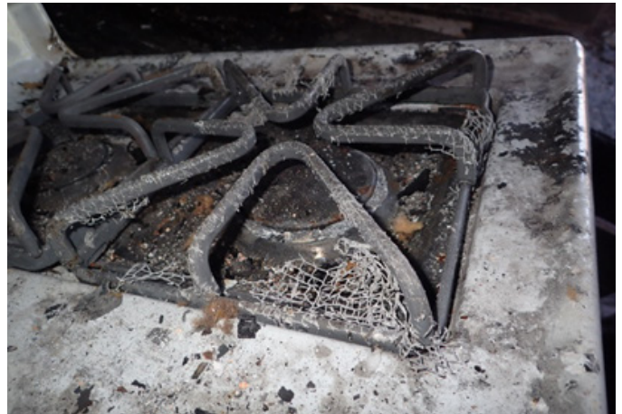
Figure 9 Mesh found on right-front burner.
