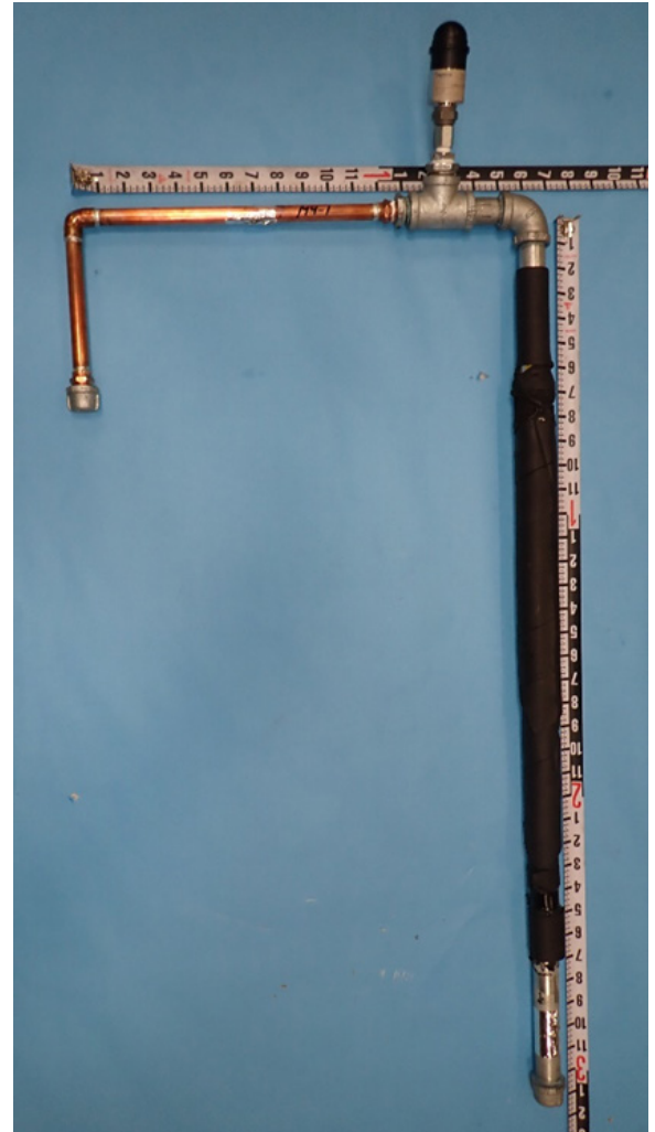
Figure 6 Photo of the galvanized pipe test apparatus, showing pressure transducer and copper tube test assembly attached. Different configurations of copper tube assemblies were tested. Accordingly, this copper tube assembly is different than the one illustrated in Figure 5.
