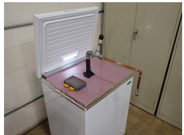
Figure 7 Photo of the test setup, showing test apparatus installed in freezer.
