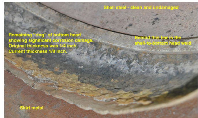
Figure 10 An image from the CSB report showing the corrosion of the 6-inch ring.
