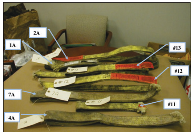
Figure 32 Sling sections retrieved from the incident site. A total of seven sections were retrieved. The Ex_Lift sling 1A, All_Lift slings 2A, 4A, 7A, #11, #12, & #13 tagged and labeled.
