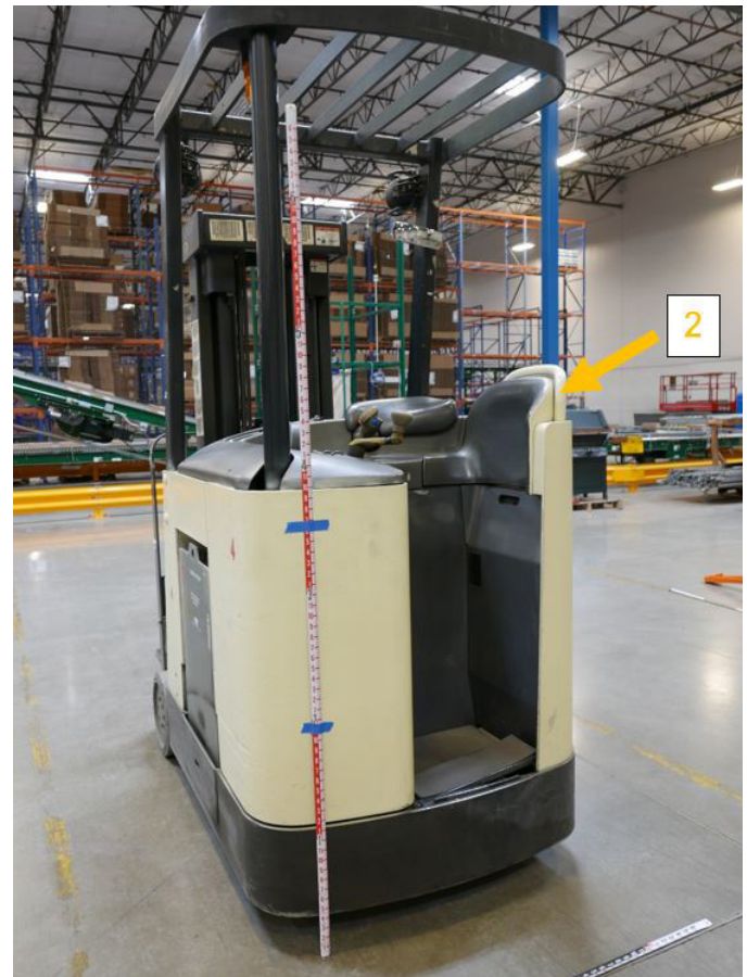
Figure 16 Stand-up forklift equipped with a horseshoe-shaped fourth corner extension feature (arrow #2).
