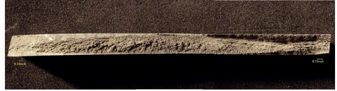
Figure 7 The fracture surface of the pipeline at the failure origin 4 . observed near the failure origin and throughout the surrounding area.
