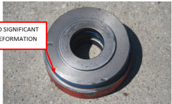
Figure 4 Inside of piston head after incident.
