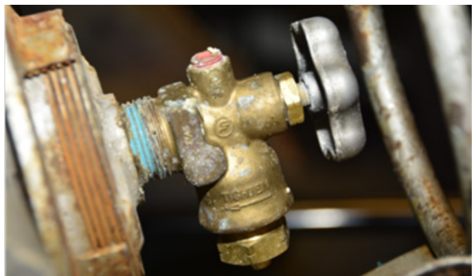
Figure 15 Left cylinder. The cylinder was ruptured, and the cylinder valve had no relief valve or fixed maximum liquid level gauge.
