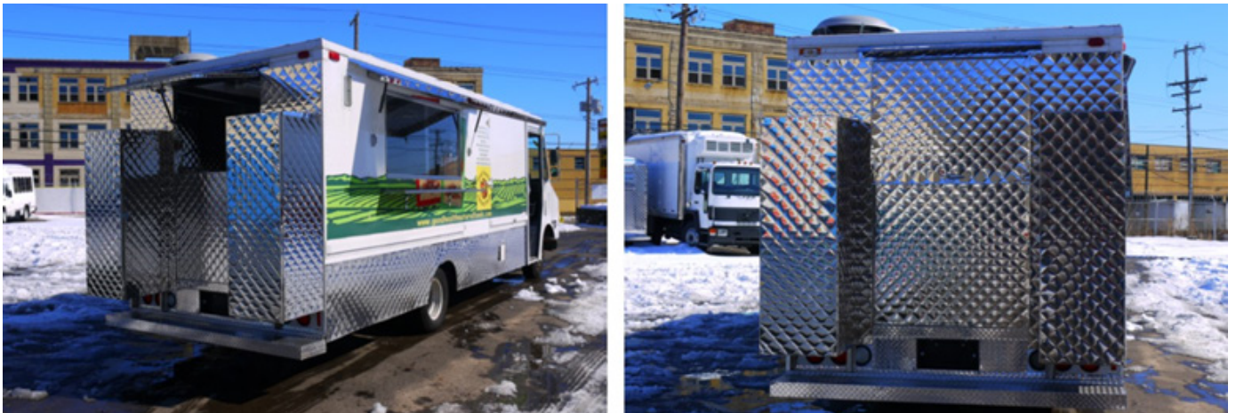
Figure 11 Pre-incident images of the rear of the food truck and the left and right propane cylinder cabinets.
