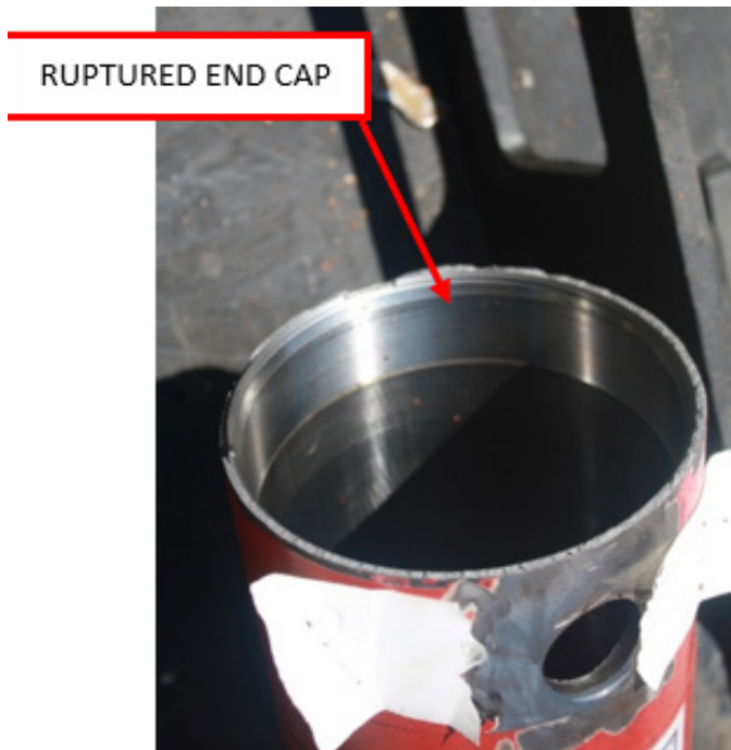
Figure 3 Cylinder end where cap was severed.
