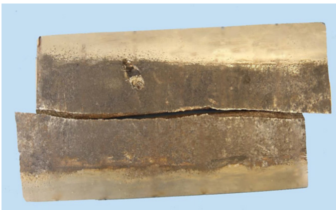
Figure 6 Sectioned segments of the pipeline at the failure origin 4 .
