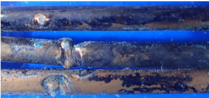
Figure 4 Example of electrical conductor arc melting damage 26 .
