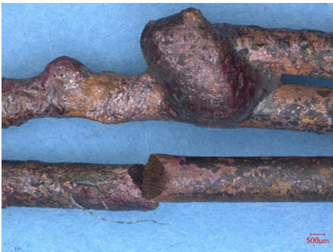
Figure 5 Example of electrical conductor fire melting damage 26 .
