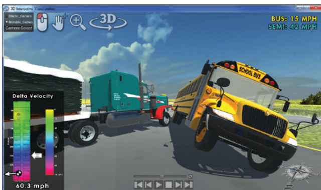
Figure 23 Interactive visualization interface displaying vehicle speeds and occupant delta velocities.
