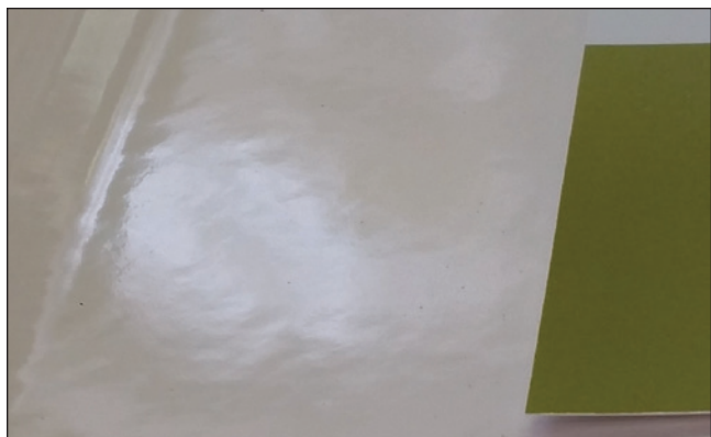
Figure 1 A new commercial “F462 compliant” porcelain enamel bathing surface with no visible texture features.
