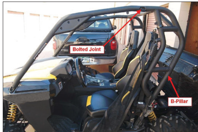
Figure 1 Undamaged exemplar UTV roll cage.
