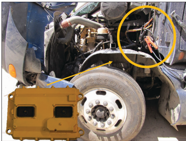
Figure 10 Power supplied through main power terminal; location of HVEDR.
