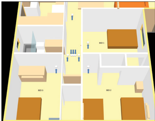
Figure 24 Hypothetical smoke detector locations.
