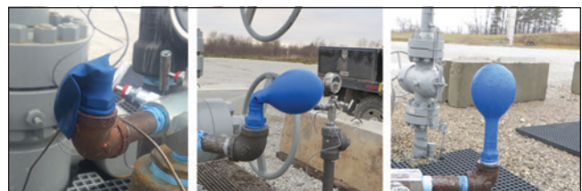
Figure 4 Photographs of different balloon test results (e.g., minimal inflation, partial inflation and upright inflation).
