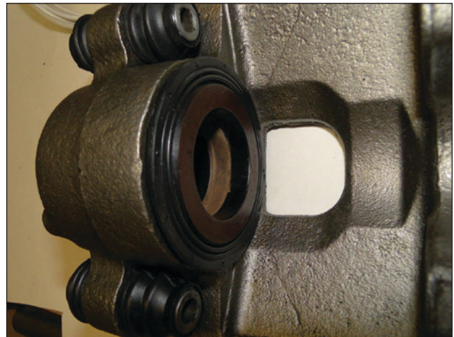
Figure 13 Exemplar caliper showing composite piston.
