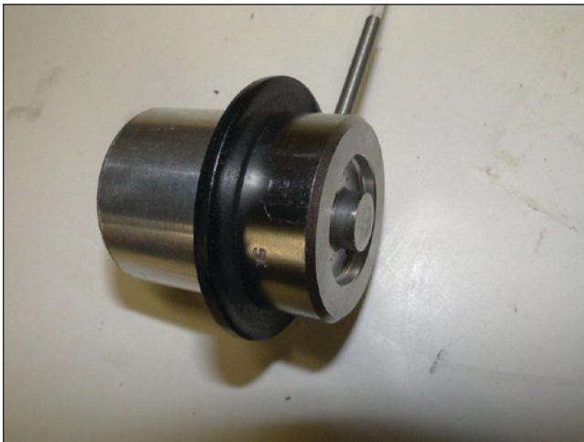
Figure 12 Mounted strain gauge.
