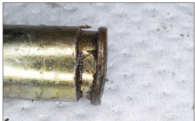
Figure 10 Deformed end of lower slider bushing.
