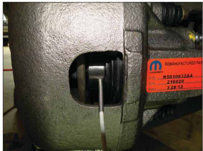
Figure 15 Instrumented caliper mounted on exemplar vehicle.
