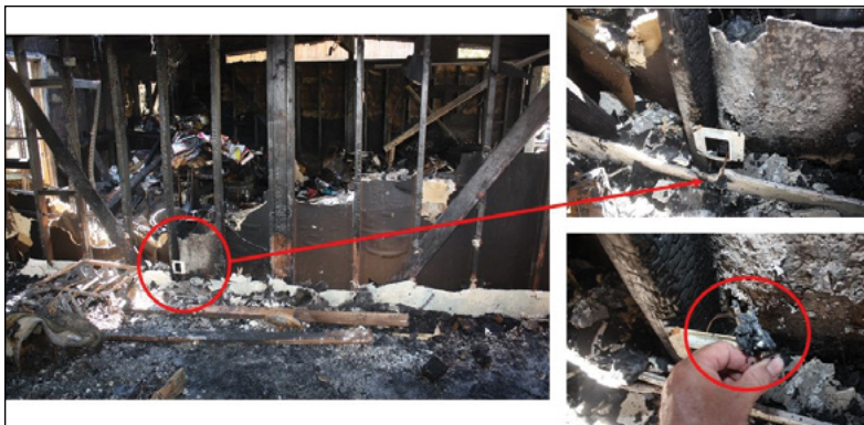
Figure 15 Evidence #2 male-female plug remains in the living room.
