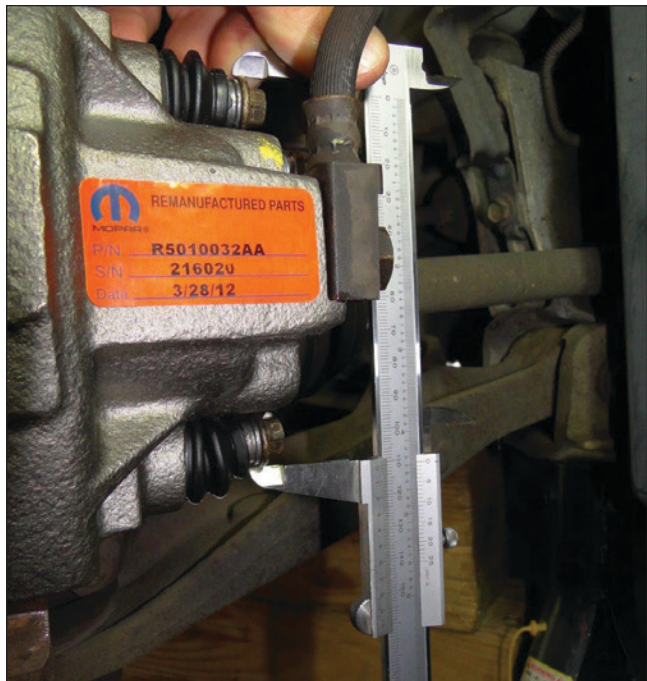
Figure 17 Measuring amount of bend.
