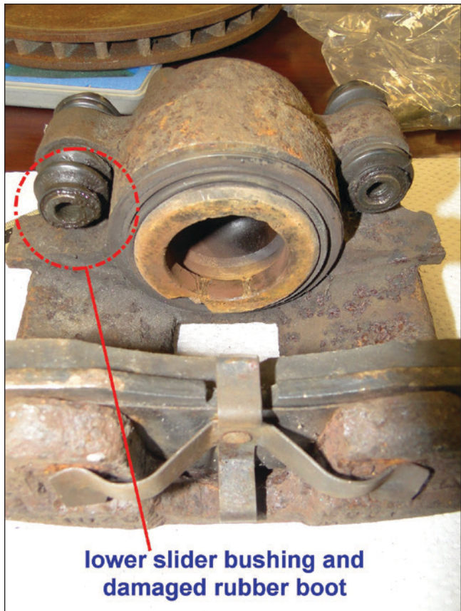
Figure 5 Lower slider bushing and boot.
