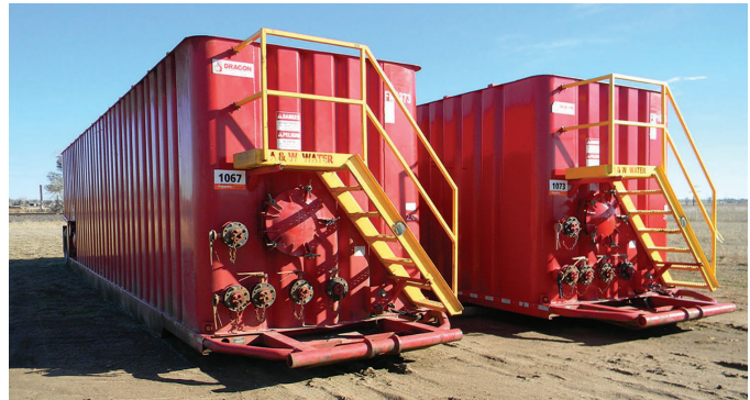
Figure 1 Typical front view of fracking tanks.
