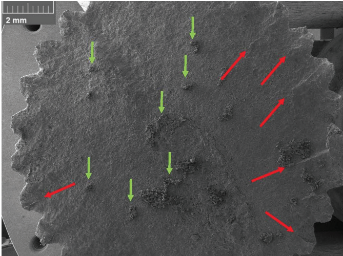
Figure 10 SEM photograph of stud fracture surface.
