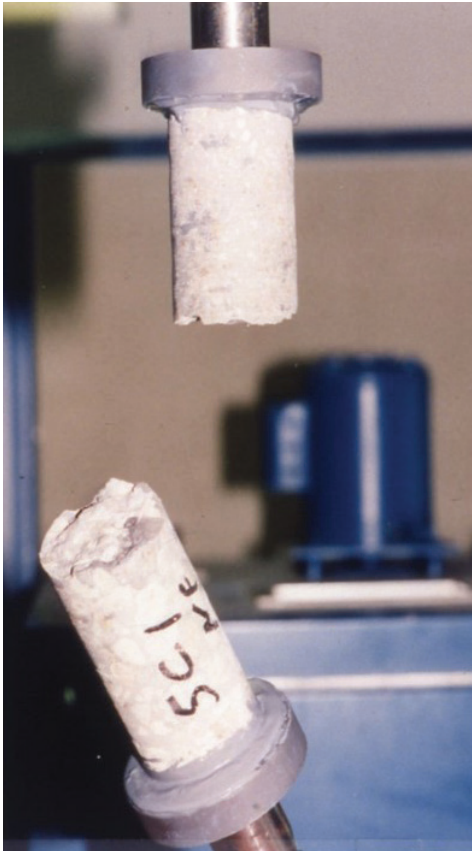
Figure 8 Tensile strength tested core.
