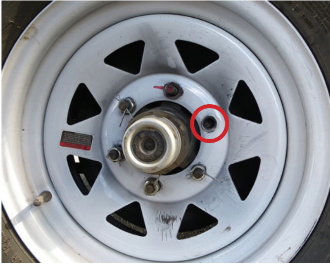
Figure 19 Trailer wheel directly after first stud fracture showing the position of the fractured stud.
