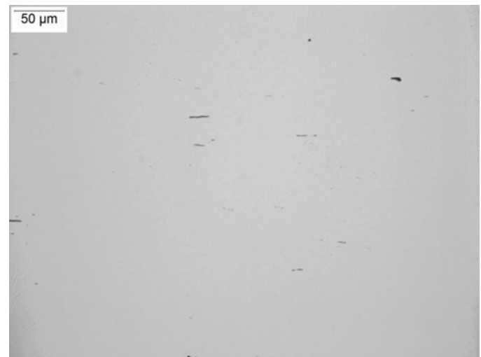
Figure 12 Metallographic sample of representative stud to examine inclusions.
