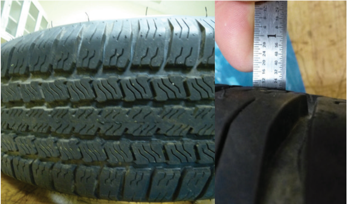
Figure 8 Accident trailer tire showing manufacturing sprues and deep tread.
