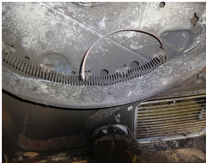
Figure 36 Bra underwire welded to heating element.
