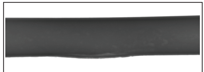
Figure 16 X-ray image of failure point bulge.
