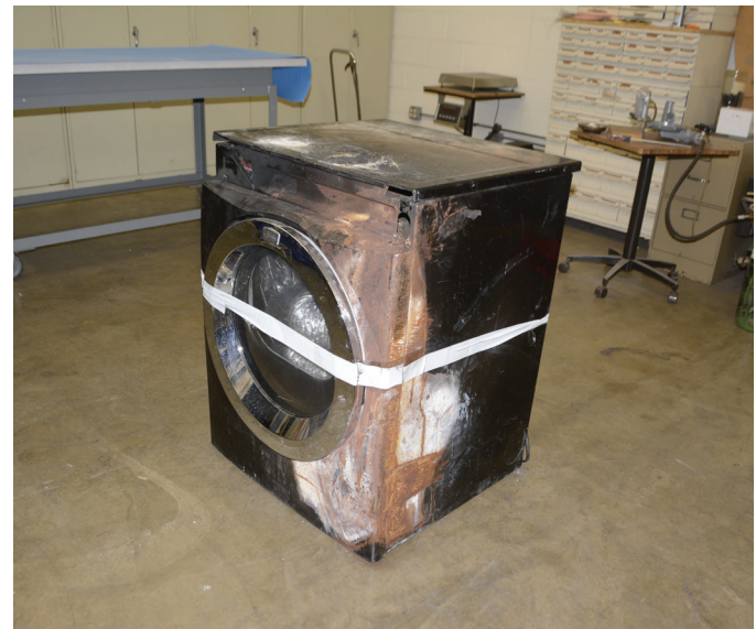
Figure 28 Dryer cabinet showing thermal damage from plastic fuel load.
