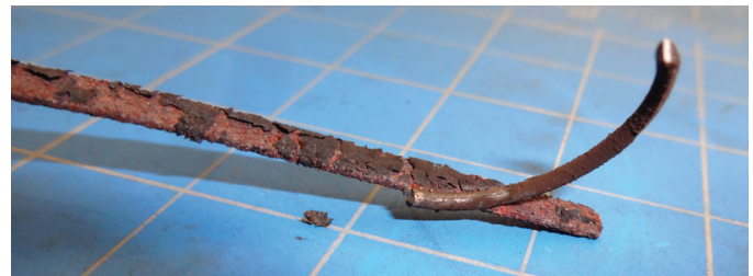
Figure 37 Bra underwire welded to heating element.
