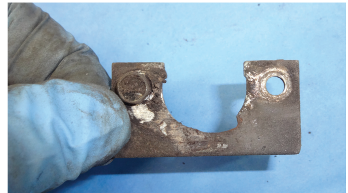
Figure 33 Wear on bearing bracket.
