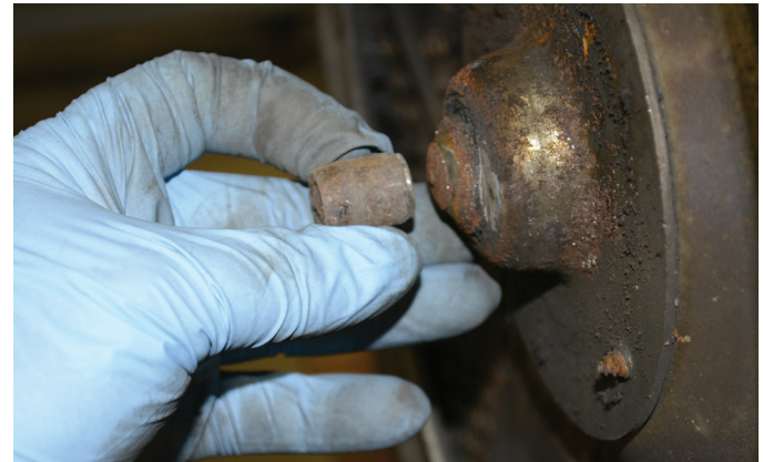
Figure 32 Severed ball hitch.
