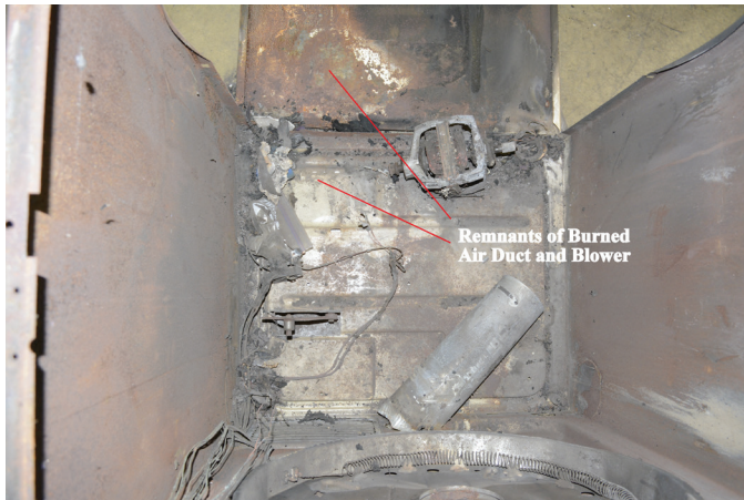
Figure 35 Consumed plastic components.
