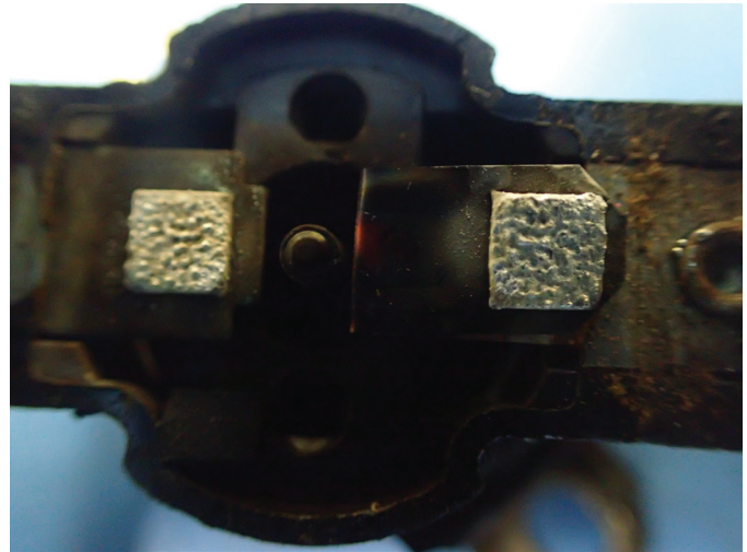
Figure 15 Contacts of electric dryer safety thermostat.
