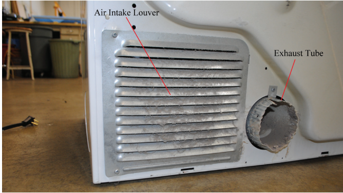
Figure 21 Exhaust tube and air intake louvers.
