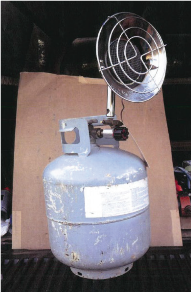
Figure 6 “Exemplar” 20-lb propane cylinder with top-mounted heater of the general type observed by the assistant fire chief and first-in firefighter.
